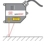
Mount the sensor only to the existing holes on a flat surface. Clamps of any kind are not permitted. Do not exceed torques. The laser beam must be directed perpendicularly onto the surface of the target. In case of misalignment it is possible that the measurement results will not always be accurate
