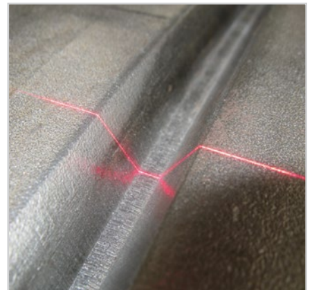
V-gap measurement on pipes
