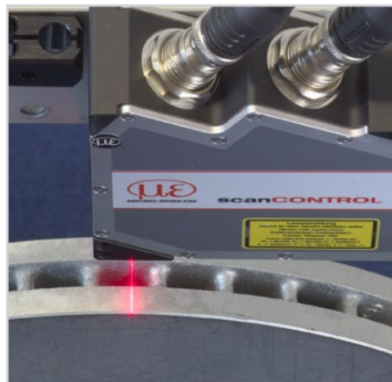
Profile measurement of the brake disc
