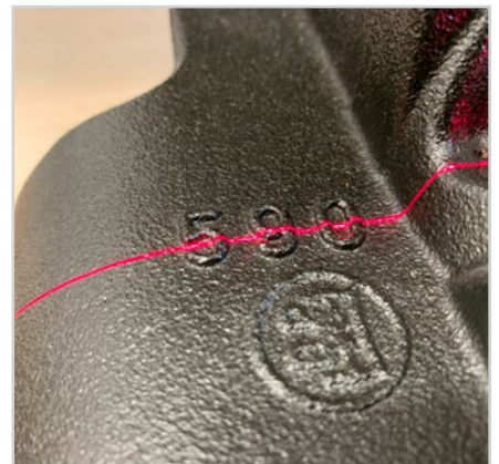
Text recognition on the cast part
