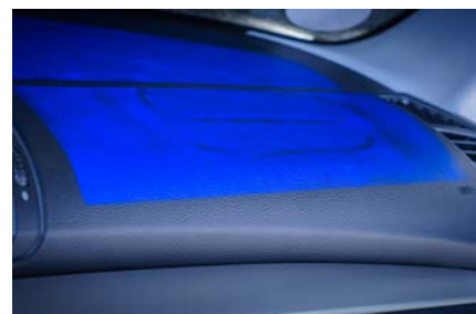
Full-surface back projection of the inspection result
