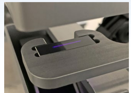
Fully automatic calibration enables reliable measurements (here: thicknessGAUGE.laser profile)
