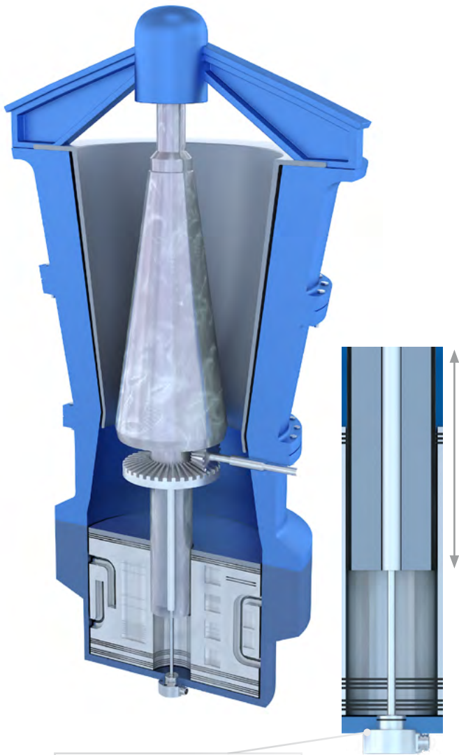
EDS-F: Measuring the grinding gap in crushers
