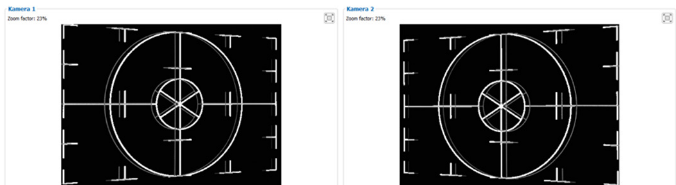
Fig. 21 Distance too large (4 mm under the zero plane)
