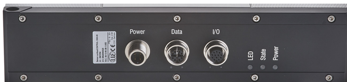
Fig. 10 Arrangement of connections
